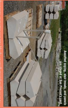
concrete or mortar cast into blocks or small special molds so as to esemble natural building stone."
